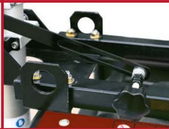
MAST SUPPORT AND FOUR RINGS FOR LIFTING
